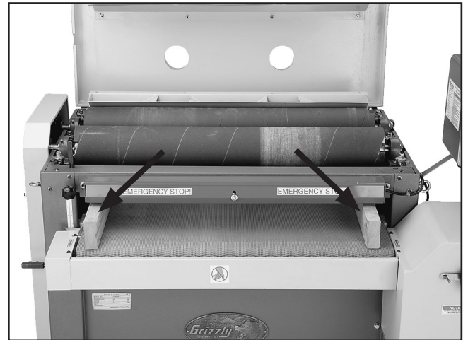
Figure 40. Gauge blocks in position for adjusting the pressure roller height.
